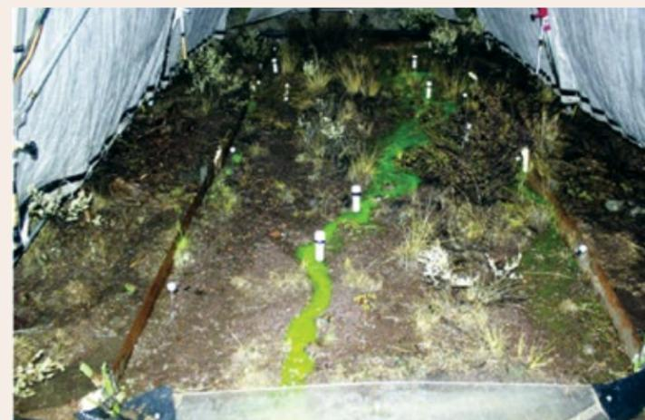
▲ Figure 5: A green dye was added to the runoff flow to emphasize creation of a concentrated flow path. Ground cover is important to slowing the movement of water to increase the opportunity for soil infiltration and decrease the risk of downstream flooding. (Source: USDA/ARS/Northwest Watershed Research Center)
